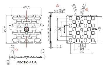
Dimensions with unmarked tolerances refer to GBT14486 tolerance table.
