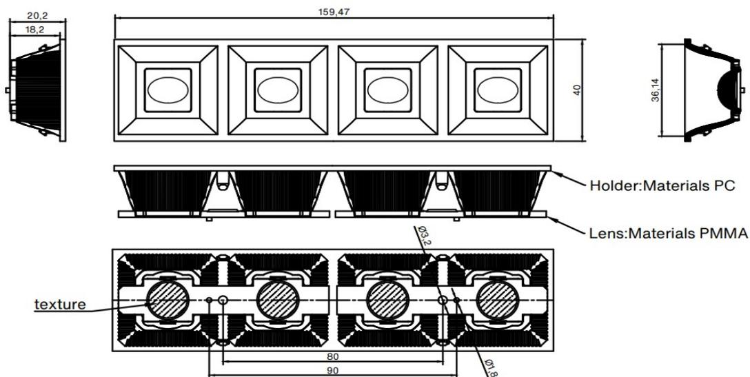
Dimensions with unmarked tolerances refer to GBT14486 tolerance table.
