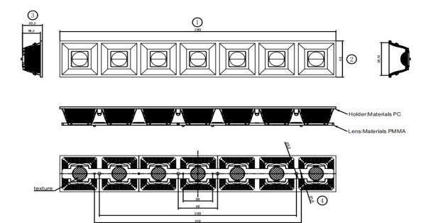
Dimensions with unmarked tolerances refer to GBT14486 tolerance table.
