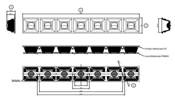
Dimensions with unmarked tolerances refer to GBT14486 tolerance table.
